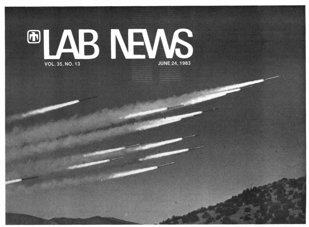
THIRTEEN-ROCKET SALVO above flies toward a target with no significant interference among the rockets. Before the launch (right), the rockets were arranged in a concentric cluster. A computer model of trajectories led to a firing sequence that minimized in-flight interference but allowed all 13 to strike the target simultaneously.
